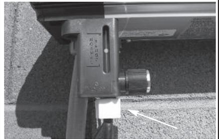
5. Lay the 3/8 tubing along desired route to the compression fitting on the combination needle valve flow meter on the Clear O3® unit.
